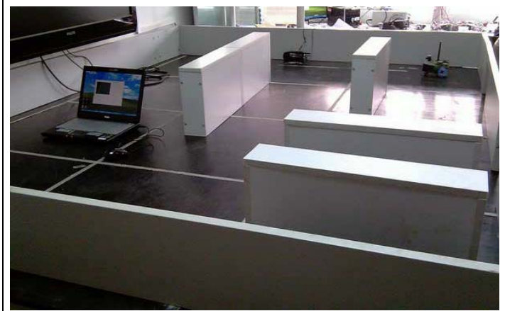
Fig.10. Testbed setup for the automatic docking experiments.
